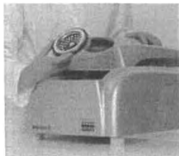
Placing a 72-Well Rotor into the Rotor-Gene Q.
