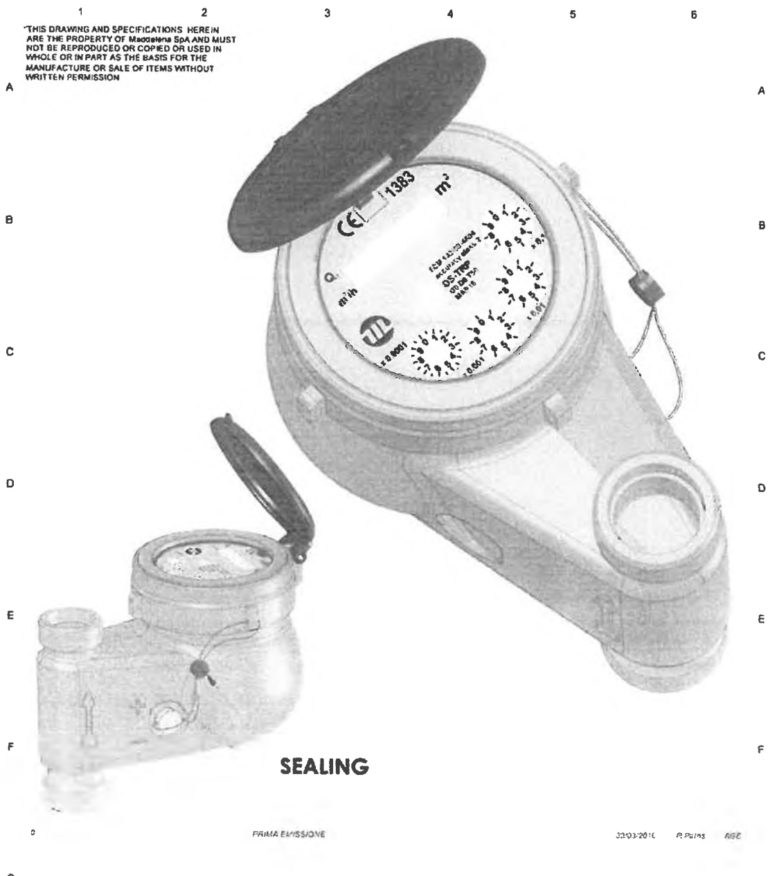
Figure 4: The body for vertical version and sealing of the DS TRP water meter
